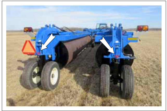
FIG. 37 TAIL WHEEL LOCK PINS
