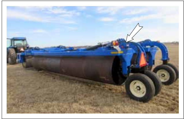
FIG. 39 TAIL WHEEL ASSEMBLY LOCK PIN (TYPICAL)
