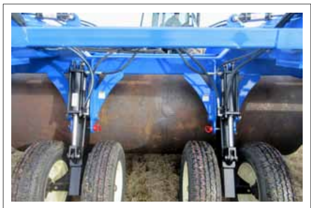
FIG. 38 CENTER WHEEL ASSEMBLY LOCK PINS
