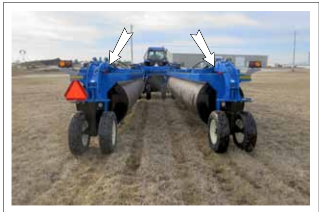
FIG. 20 REAR WHEEL LOCK PINS STOWED
